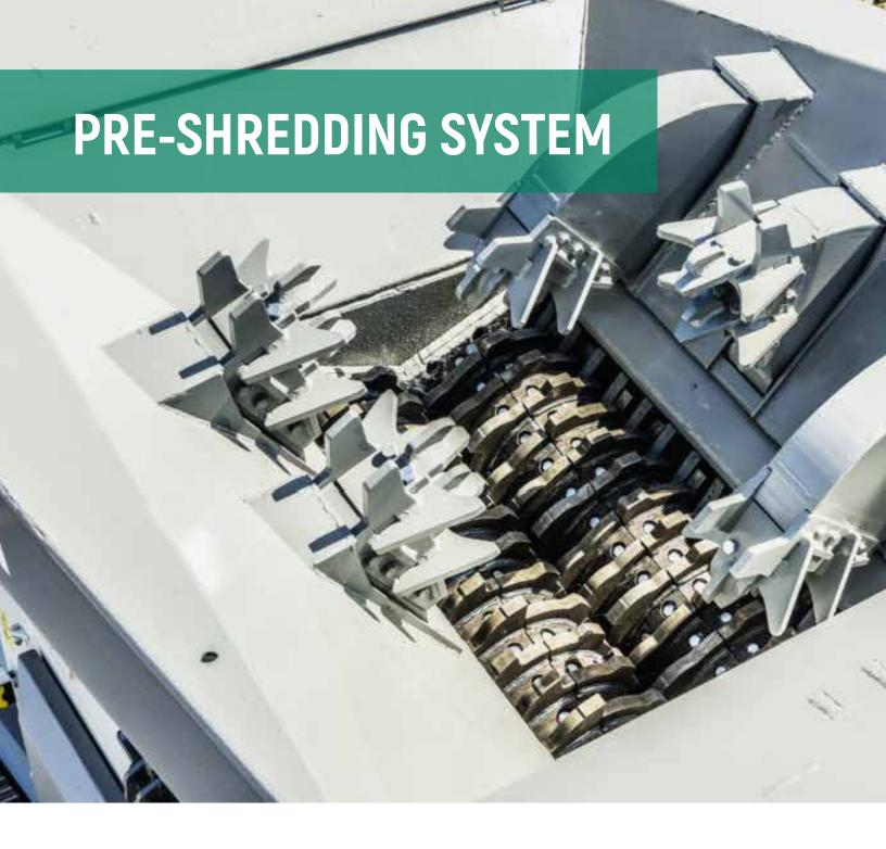
The patented  $CAMS^{TM}$  hydraulic pusher system allows even the largest blocks to be loaded directly into the shredding unit.
