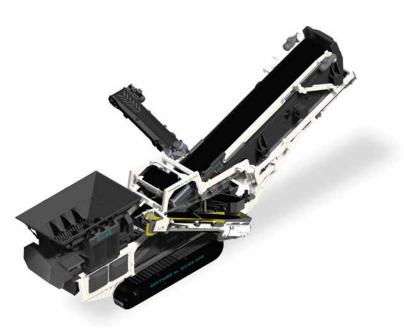
**Hopper** Capacity: 3.80 m<sup>3</sup> Length: 3.50 m Width: 2.00 m
